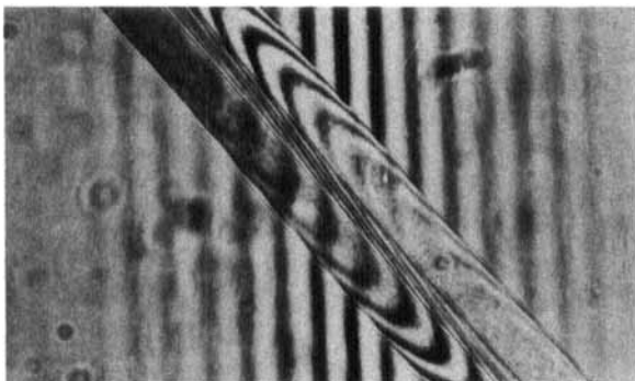
FIGURE 2 Totally duplicated image of the fiber using white light vibrating parallel to the fiber axis.
